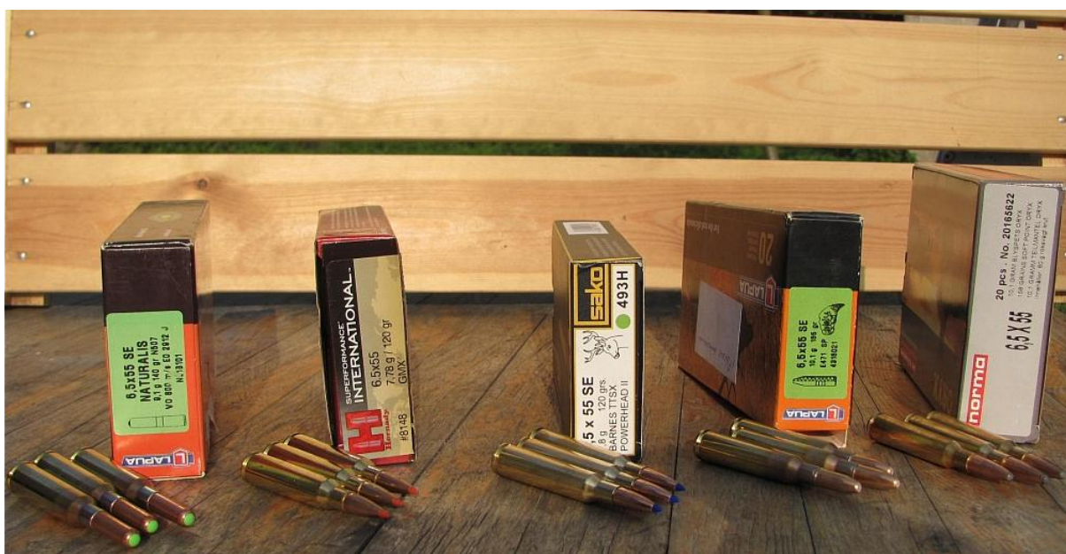
Figure 1: The tested 6,5x55 SE ammunition. Lapua Naturalis (Lead free), Hornady GMX (Lead free), Sako Powerhead II (Barnes TTSX Lead free), Lapua Mega, Norma Oryx (Bonded)
