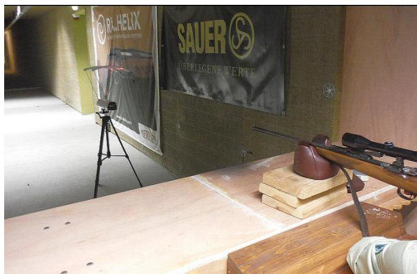
Figure 3: Test rifle at indoor range with Chronograph set up to measure starting velocity ( V_3 ).
