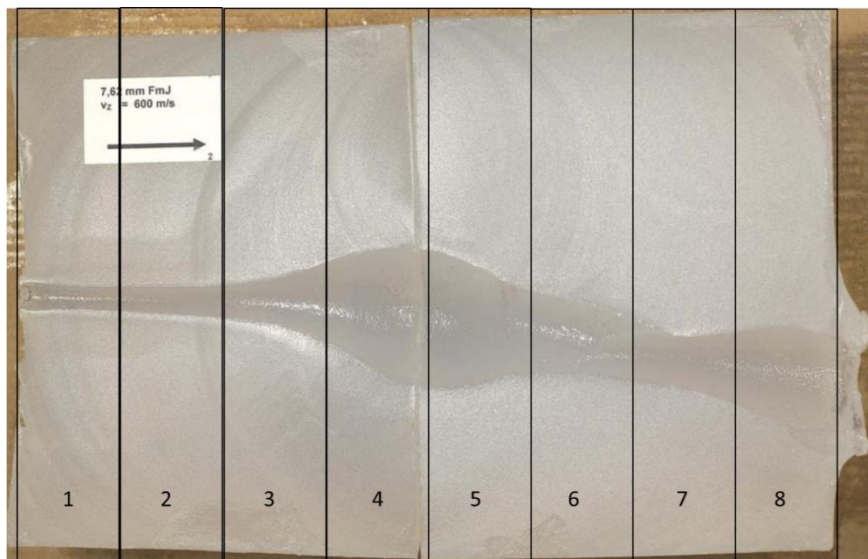
Figure 7: Example for 5 centimeter segmentation of the soap block. Entrance of this .308 Win. Full – Metal – Jacket –Bullet (FMJ) bullet was from the left.
