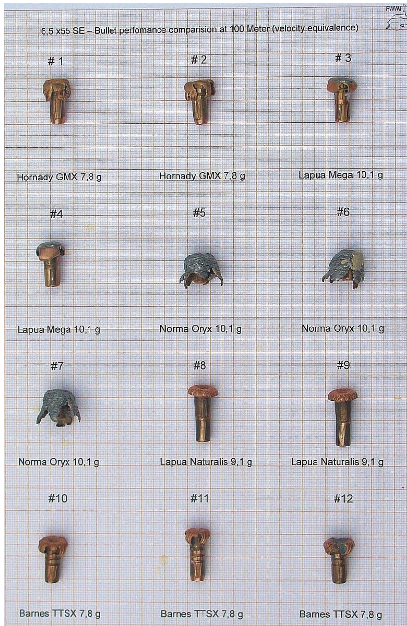
Figure 9: Photograph of bullet bodies (side view) after traversing the soap block. All but shot # 12 (stopped at 38 cm) exited the block.
