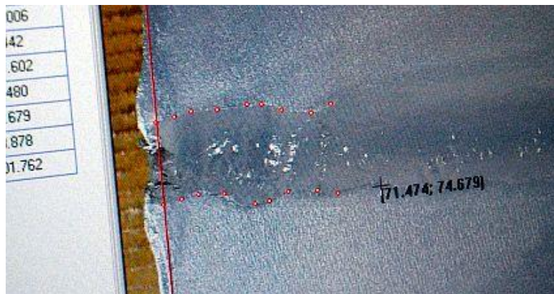
Figure 6: Representative picture of measurement of a cavity produced inside the soap block at the PC using a scaled photograph.
