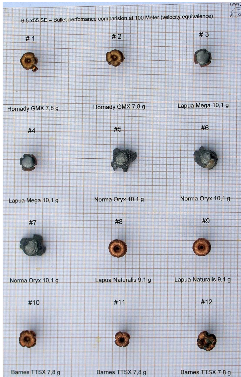
Figure 8: Photograph of bullet bodies (frontal view) after traversing the soap block. All but shot # 12 (stopped at 38 cm) exited the block.
