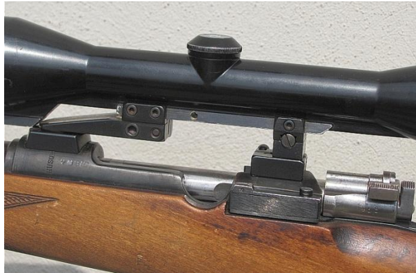
Figure 2: Test rifle Husqvarna M38, build in 1942, with EAW Pivot Mount and Zeiss 6x42 Scope.
